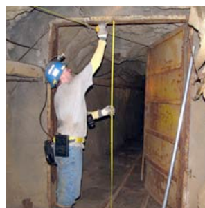
Left: Bruce Pietzyk performs ventilation check at Yates air door
